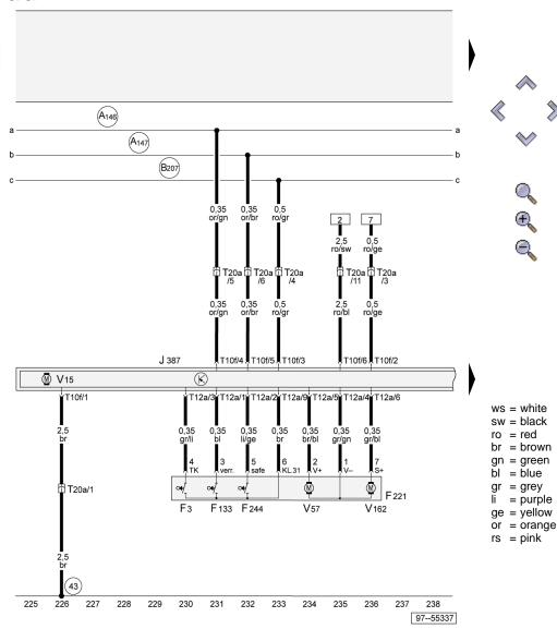
Door control unit (front passenger's side) with electric windows, central locking lock unit (front passenger's side)
