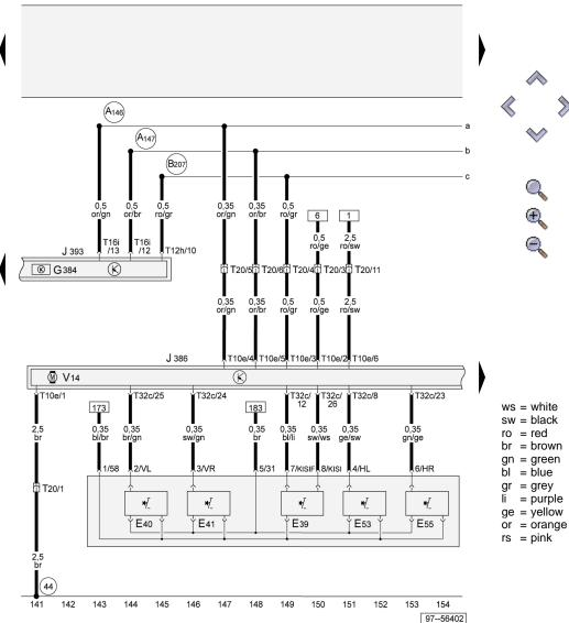
Convenience system central control unit, door control unit (driver's side) with electric windows, electric window switches, vehicle inclination sender
