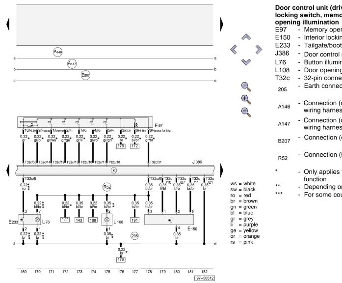
Door control unit (driver's side) with electric windows, interior locking switch, memory operating unit (driver's seat), door
